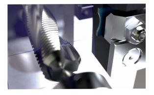
Alignment stop made of cheap rectangular symmetrical plates with a quick change system. The stop plate can be rotated to use all edges until worn.
